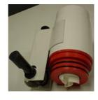
These pictures show the waste pump as used in the Wet Floor Kit and Corner Cubicle. Float switch at 90 deg. Available in two voltages, 24 and 12. Check voltage on wiring block label if unsure.
