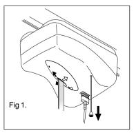
The red pull cord provides an emergency cut out. If the cord is pulled once then the emergency stop is activated. To reset, pull the short piece of cord located on the top face of the hoist. Proceed to press the red reset button located on the handset. Three beeps sound when the hoist is then reset and ready to use.
