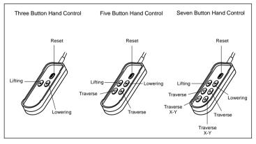
Please Note: The handset is the correct way round when the cable is at the top.
